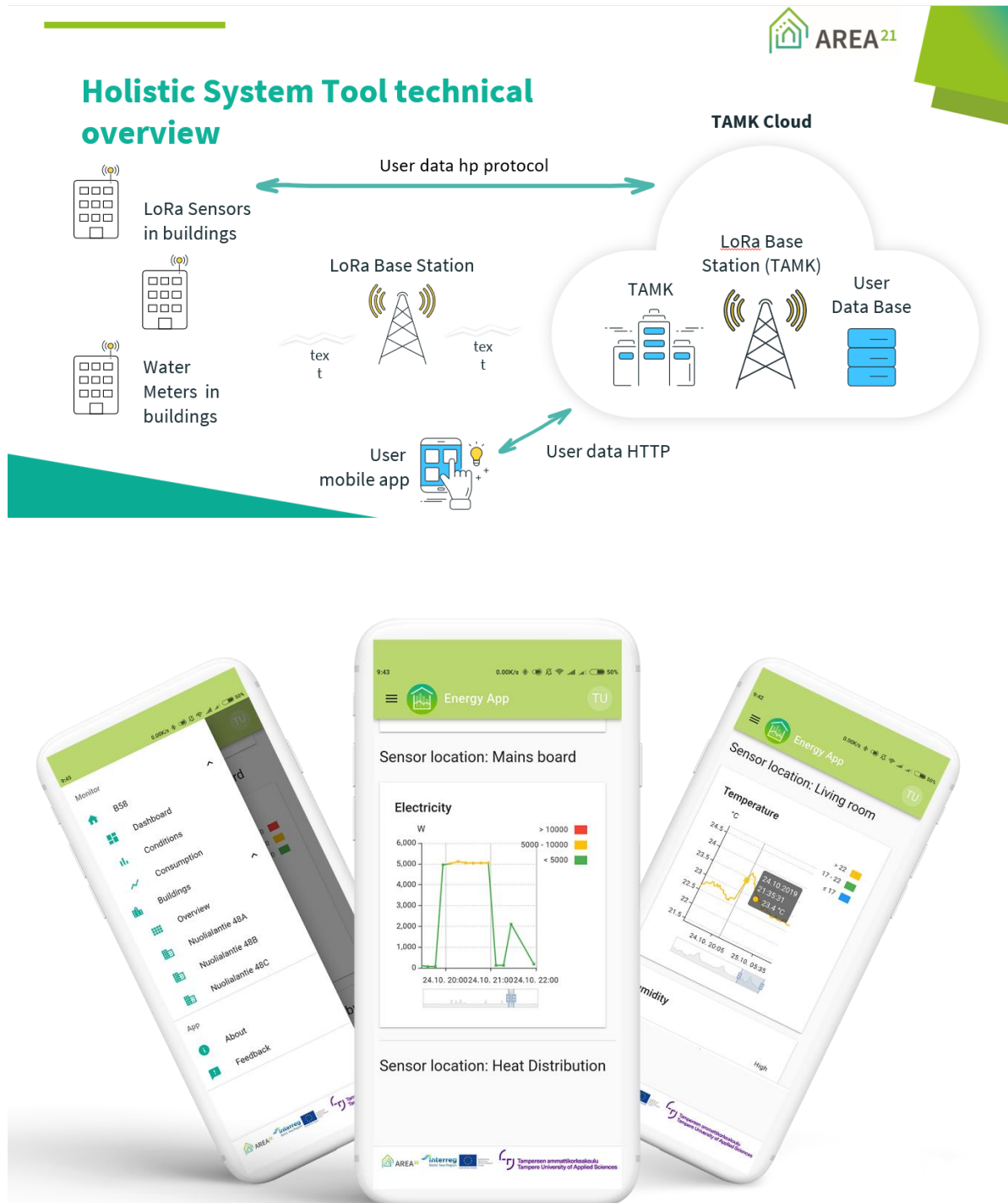
Figure 2. The system overview and mobile application interfaces of the real-time energy monitoring tool (Source: AREA 21 project)
