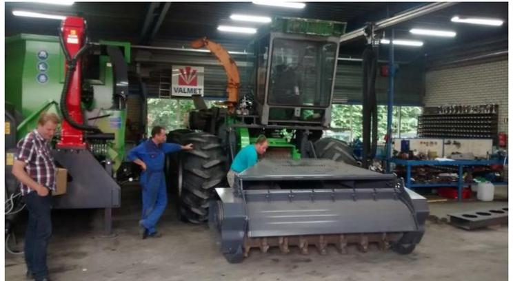
After the in-house test, the machine was field tested in the estate “De Treek” in the Netherlands (see picture). During the field test it appeared that the machine was not working optimal yet, and that further developments were required. In addition, the weight of the machine (10 tonnes) appeared rather high in light of its intended application. This can be problematic on sensitive forest soils.
